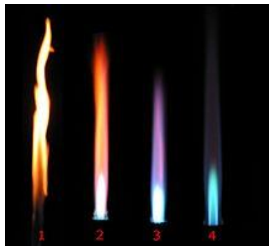
Figure 7: The left is a rich fuel mixture with no pre-mixed oxygen, producing a sooty diffusion flame. On the right is a full oxygen premixed flame, producing no soot [6]
