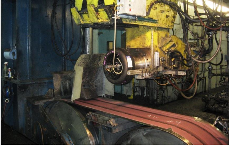
Figure 4. F&M testing at the Calspan Tire Research Facility. Photo from FSAE TTC.
