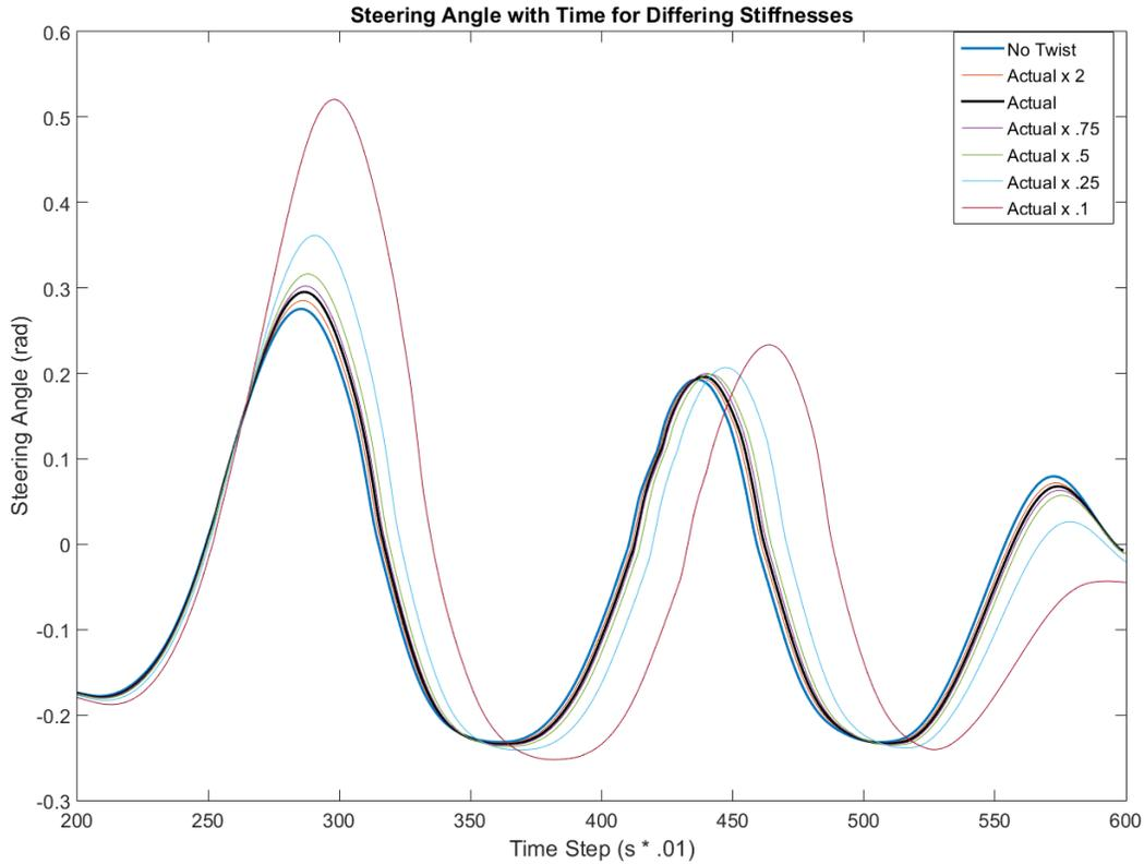
Figure 4: Steering angle is shown against time for the wide J-turn event for vehicles of varying chassis torsional stiffnesses.
