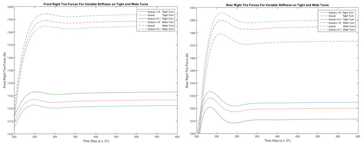
Figure 2: Front and rear outside tire normal forces for tight and wide turn at various stiffnesses where Actual stiffness refers to 2100 Nm/deg.
