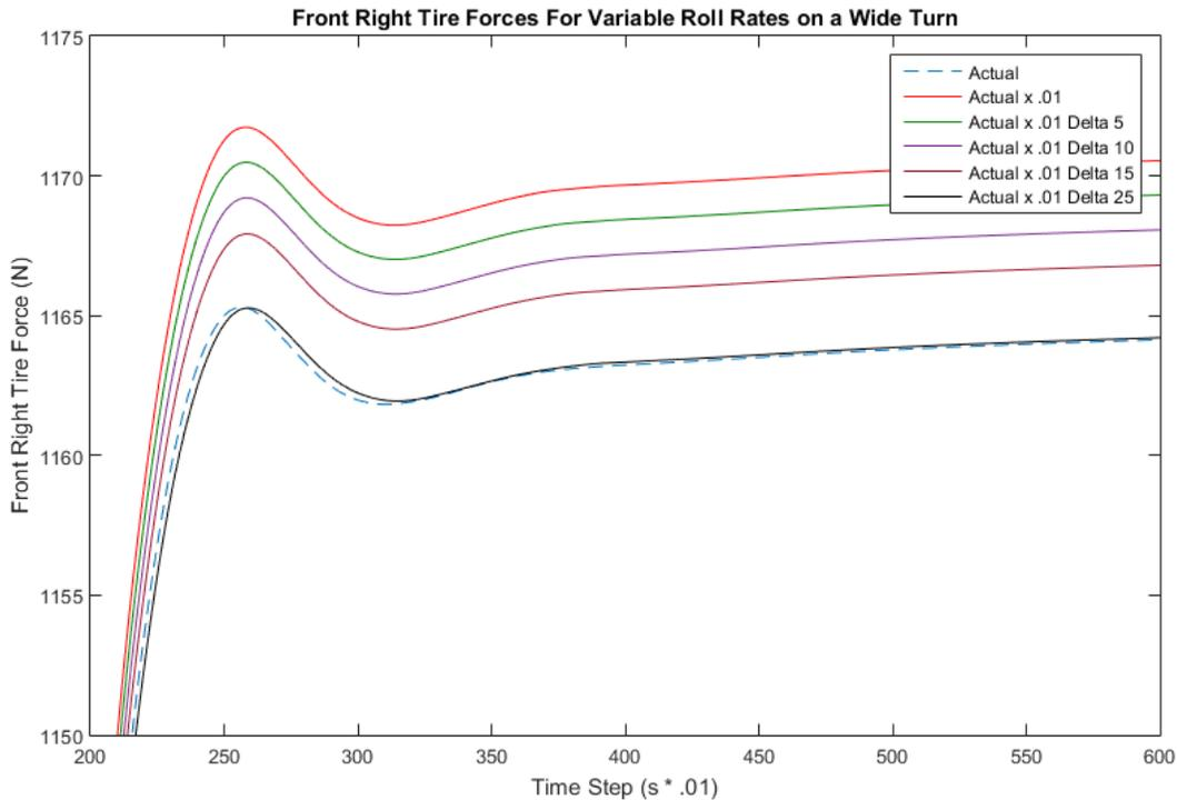
Figure 3: Front outside tire normal forces for chassis of various chassis torsional stiffnesses and of various suspension spring rates. Where Delta # refers to a # lb/in spring rate decrease in the front springs and # lb/in increase in the rear springs.
