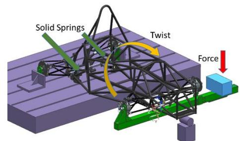
Figure 1: Chassis stiffness physical test setup
