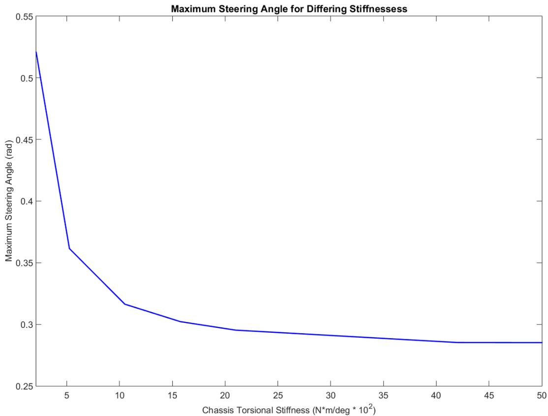
Figure 5: Maximum steering angle in the wide J-turn event against chassis torsional stiffness
