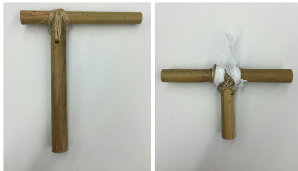
A.. Simple right angle joints lashed with twine and plastic bags
