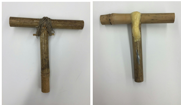
A.2. Prototypes for Epoxy reinforced joints. It was later decided that epoxy was not locally obtainable. It was therefore ruled out as a building material.
